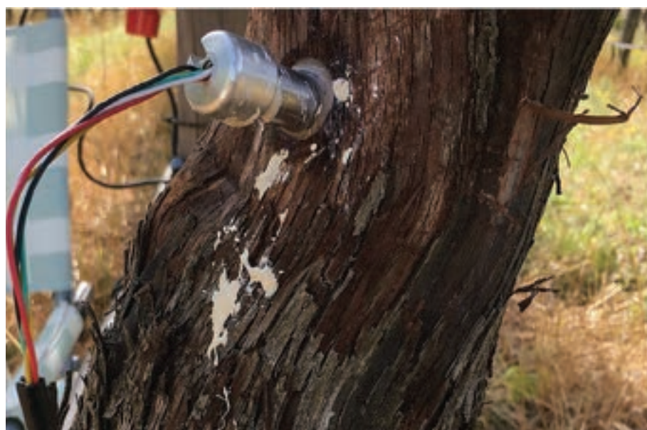
FIGURE 3: An installed FloraPulse microtensiometer on a grapevine
