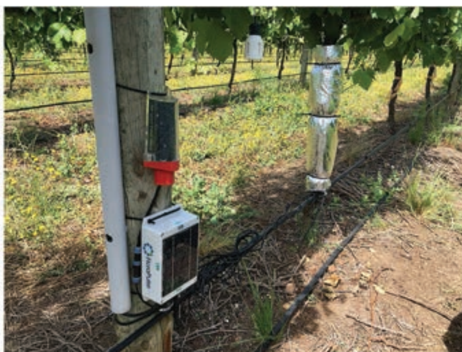
FIGURE 4: A FloraPulse microtensiometer installed on a grapevine with its protection materials and its connection with the data collection and transmission equipment.
