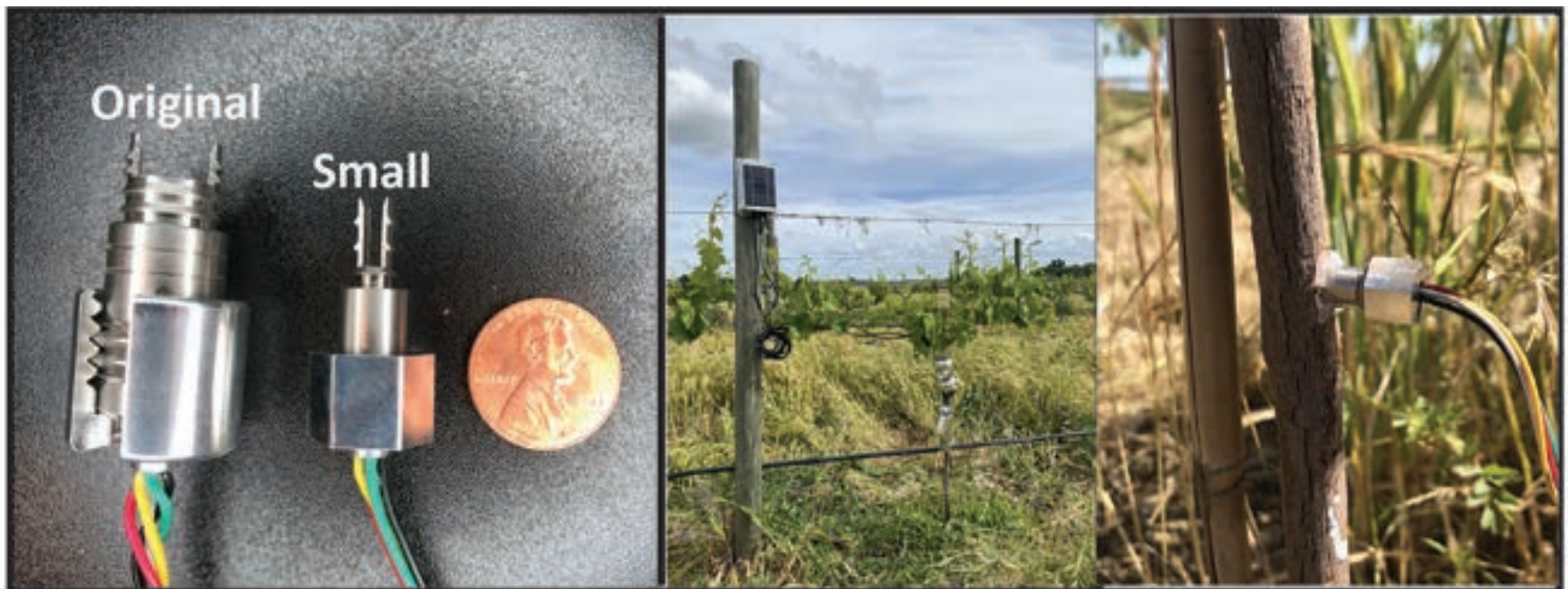
FIGURE 7: The photo on the left is the original size FloraPulse microtensiometer. The center image shows the new microtensiometer in position on a grapevine that is connected to the data transmitter. The right has the small unit installed.
