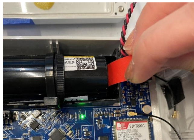
Figure 4: Use a plastic tab to cut off datalogger power for storage
